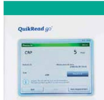
**5** The result appears on the display when the measurement is completed and the cuvette automatically rises from the measurement well.
