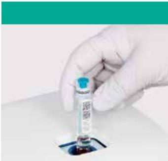
**4** Select *Measure* on the display of the QuikRead go instrument. Insert the cuvette in to the measurement well of the instrument. The barcode should be facing you.
