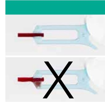
**Note!** Check that the capillary part is completely filled. **Do not wipe Sample Collector!** If there is excess sample on Sample Collector, discard Sample Collector.
