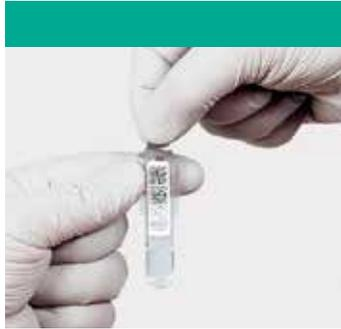
**1** Remove the foil cover from the cuvette. Do not touch the clear flat surfaces in the lower part of the cuvette.
