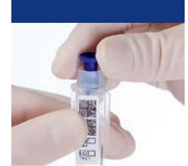
**4** Close the cuvette tightly with a CRP reagent cap. Do not press down the blue inner part of the cap. Once the sample is added to the buffer, it may be held for up to two hours prior to running the assay.
