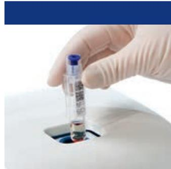
**6** Insert the cuvette in the measurement well of the instrument. The bar code should be facing you. The display shows how the measurement is proceeding.
