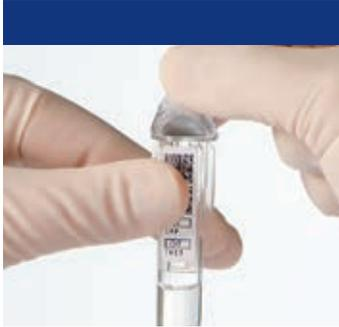
**1** Remove the foil cover from the cuvette. The liquid surface should lie between the two lines marked on the cuvette. Do not touch the clear flat surfaces in the lower part of the cuvette.
