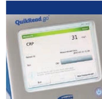
**7** When the measurement is completed, the result is shown on the display and the cuvette will rise up from the measurement well automatically. With the QuikRead go CRP+Hb test the Hb result is shown below the CRP result.
